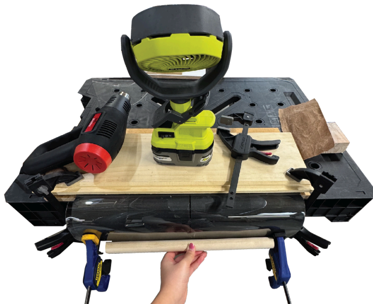
Figure 6: Heat forming acrylic with heat gun, custom PPA-CF fixture, clamps, fan, and acrylic
